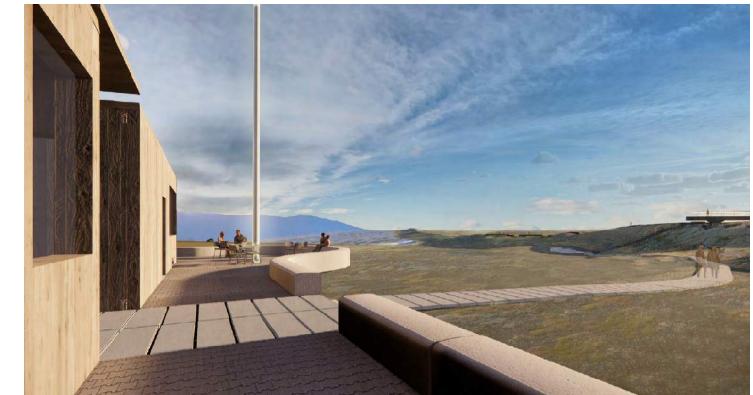
Straight and curved pre-cast concrete seating elements define the cafe terrace. These replicable precast elements can be laid out in a variety of ways that respond to the terrain
