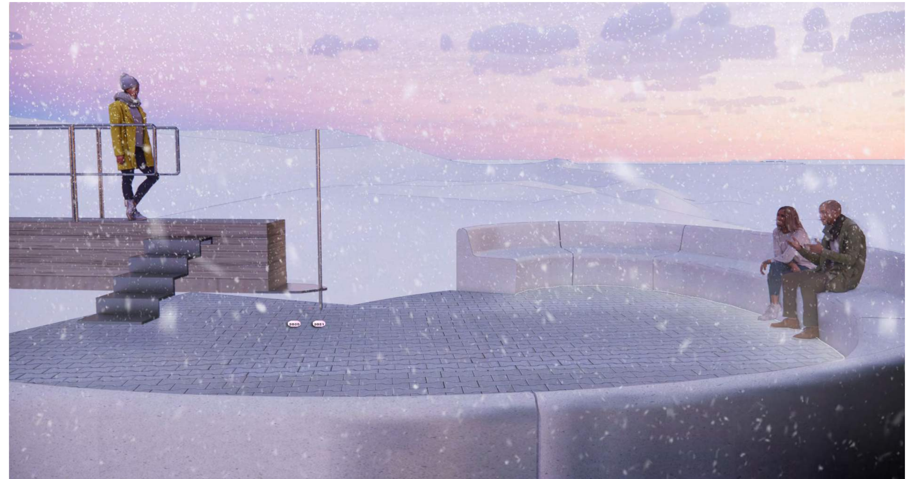
Atmospheric light of Icelandic winter when the sun hangs low on the horizon. Lighting is incorporated into the bottom of pre-cast bench elements and at the bottom of the wood beam crossing to create a low level pool of light. Radiant heat bench elements increase thermal comfort and control snow melting on the hardscape during the winter
