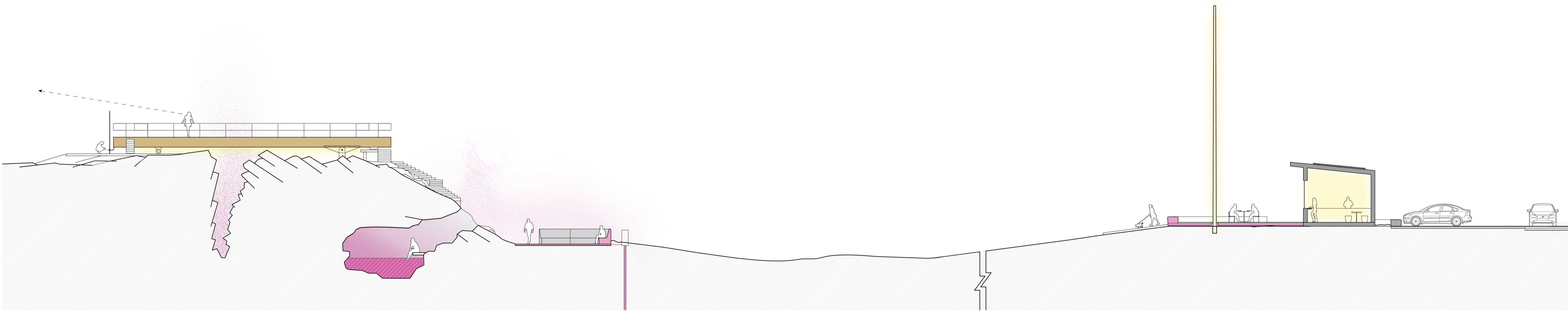
Section through the fissure showing the wood beam crossing, the geothermal bathing cave, heat island with precast concrete benches, and cafe entry building
